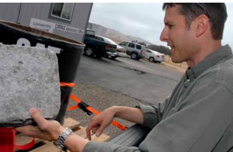
NPS student Lt. j.g. Deward Cummings holds a piece of the lightweight, fibrous concrete used in his thesis research during the latest RELIEF experimentation program in August. Cummings and Lt. Paul Mahoney are looking at developing a low-cost, fibrous concrete construction kit that can be used to safely dispose of and detonate dangerous, explosive remnants of war.
