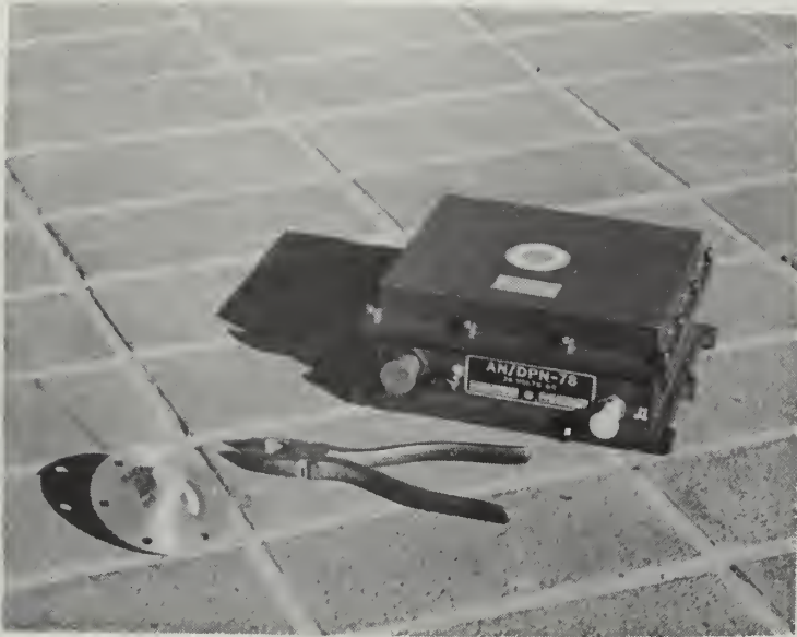
Figure 13. AN/DPN-78 Transponder and Antenna
