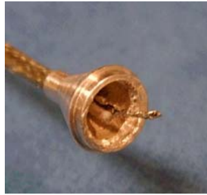
Figure 11. Cable Fitting with Silver Epoxied Braid on its Inner Walls
