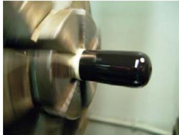
Figure 8. Hydrophone Spinning in the Lathe
