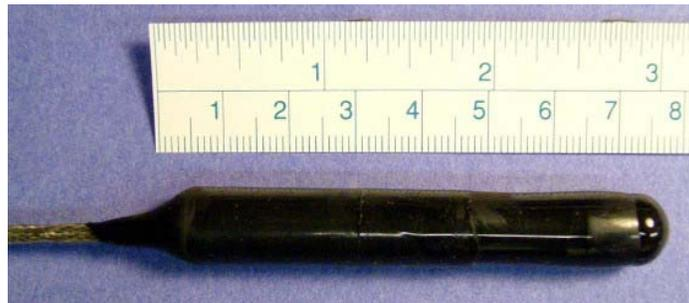
Figure 10. Hydrophone Totally Covered with Polyurethane
