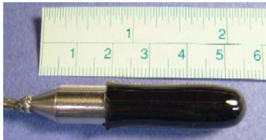
Figure 9. Hydrophone Partially Covered with Polyurethane
