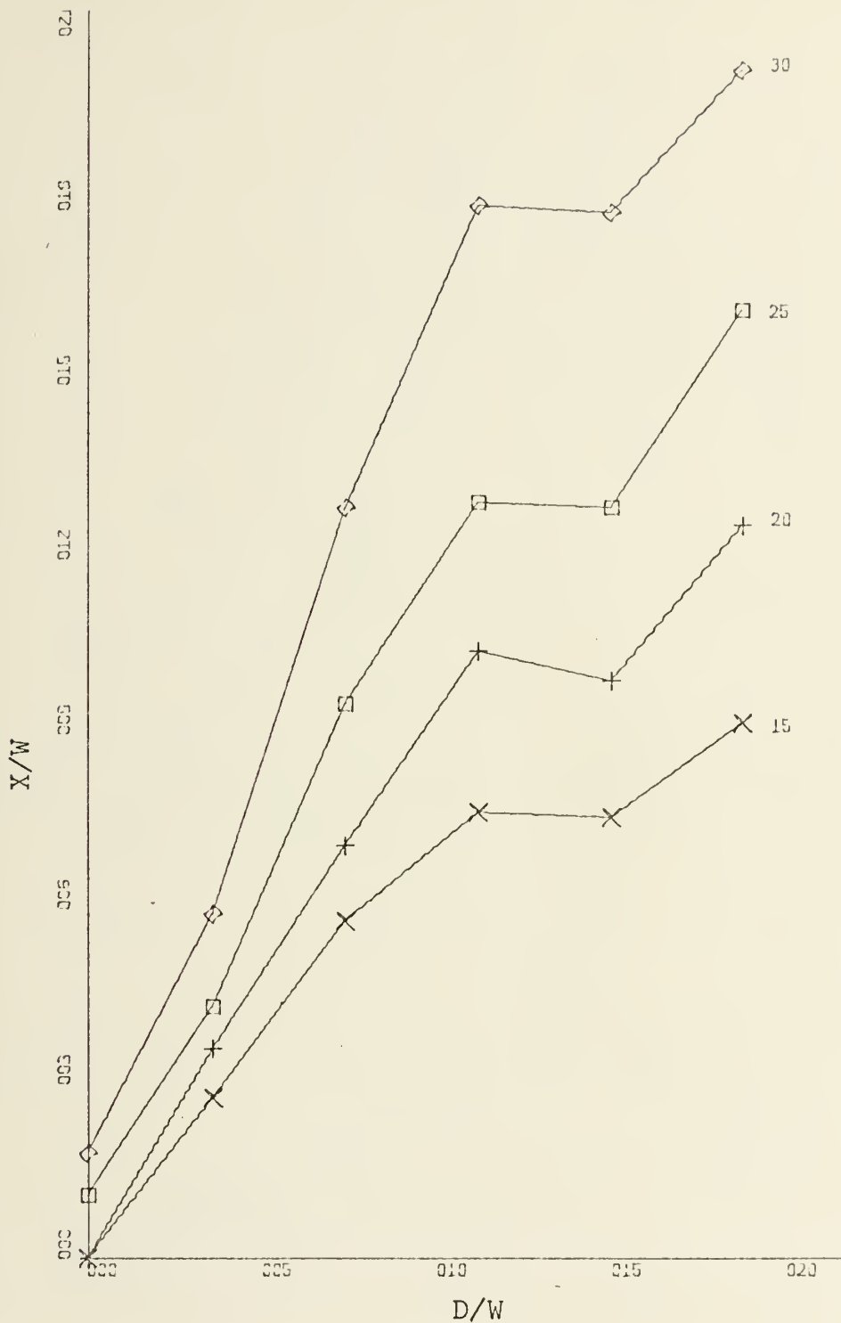
Figure 19. Attachment Distance vs. Offset Distance for Planar Wall, Re = 1.475 \times 10^5 Constant Deflection Angles of 15, 20, 25, 30 and Jet Width of 1.31 Inches.
