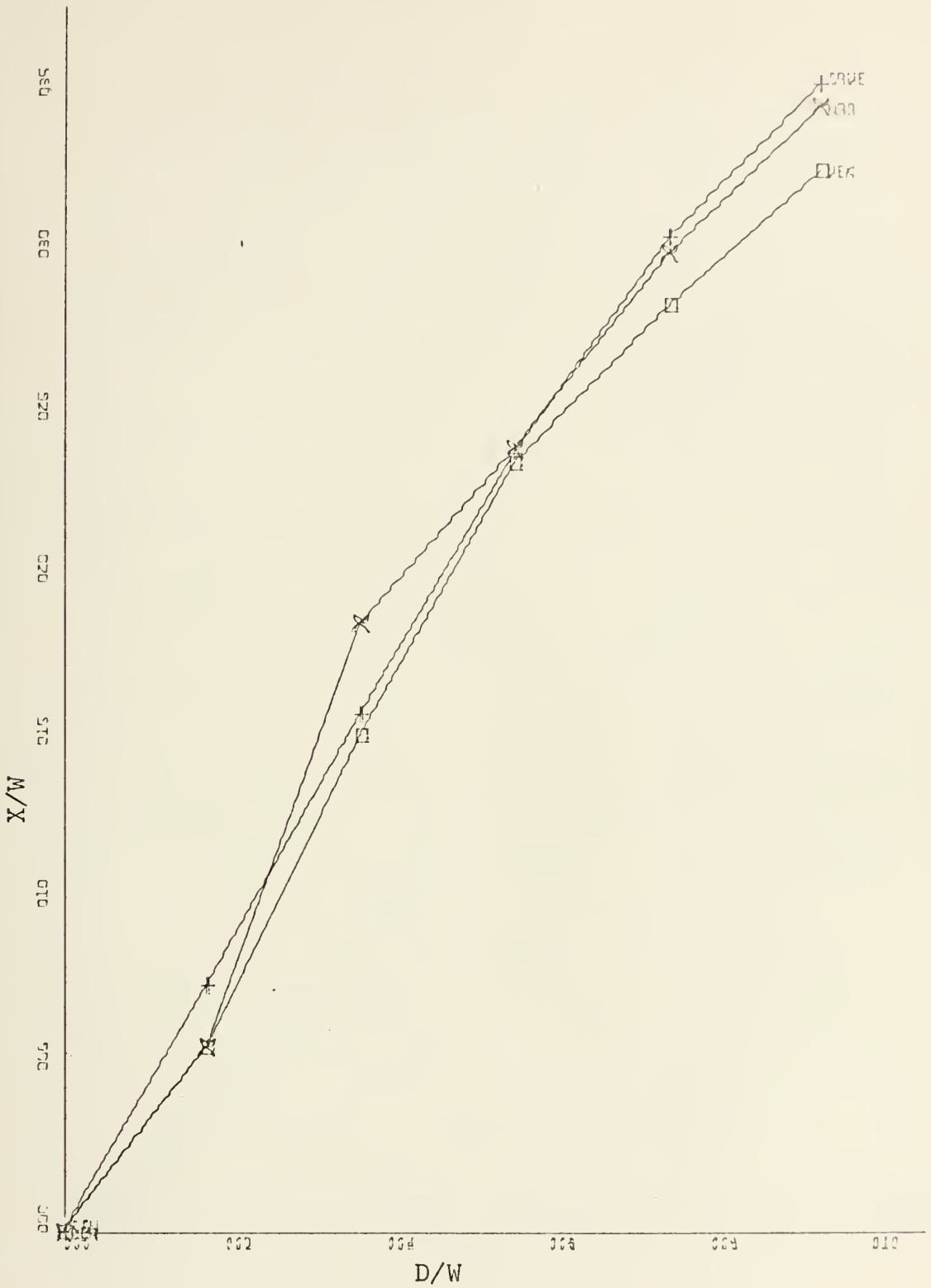
Figure 54. Attachment Distance vs. Offset Distance at 0 Degrees Deflection for Planar, Concave, and Convex Walls. Jet Width 2.62 Inches. Re = 2.05 \times 10^5 .
