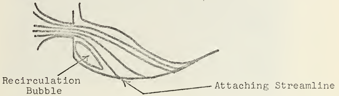
Figure 2. Flow Model for Concave Wall
