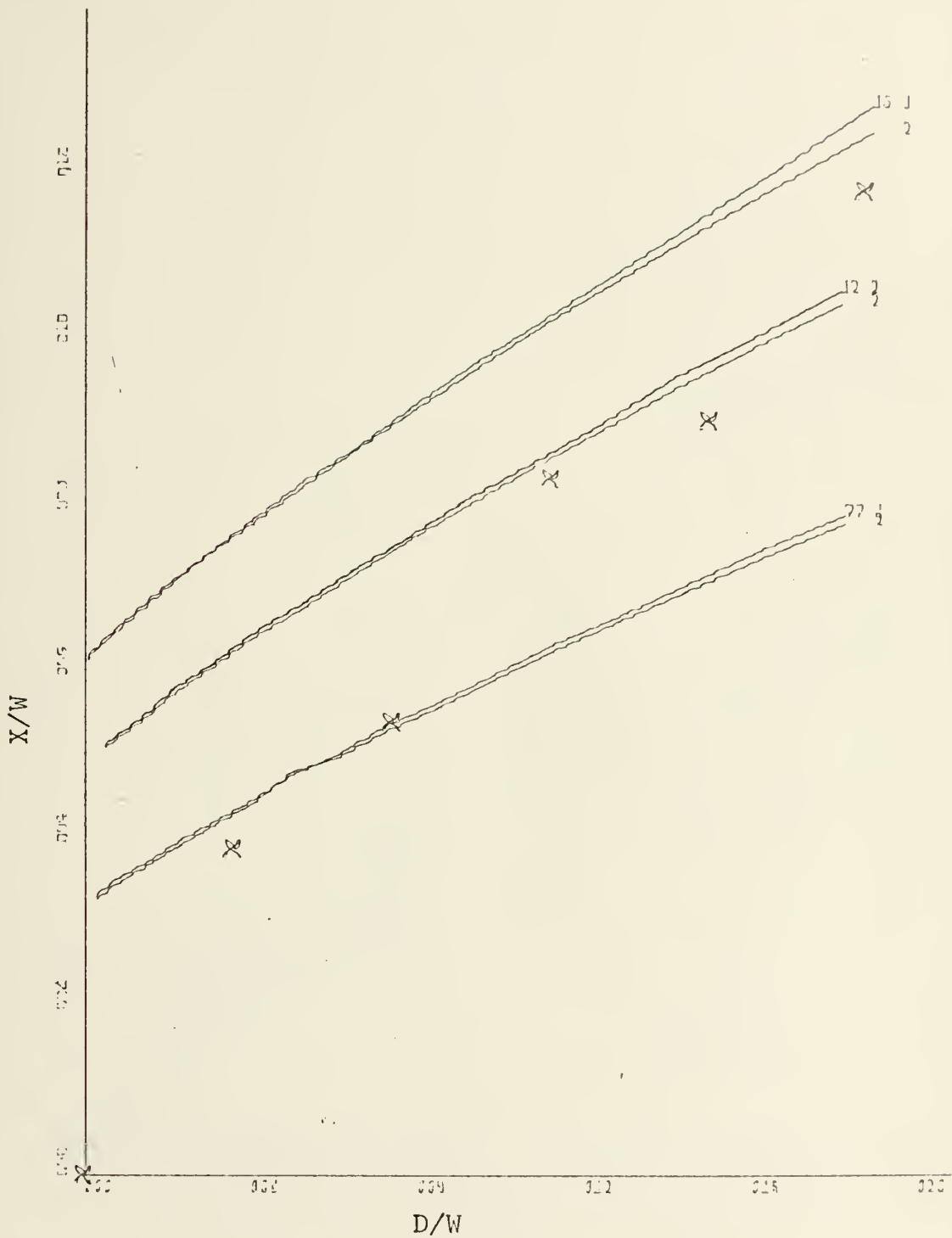
Figure 31. Attachment Distance vs. Offset Distance for a Convex Wall, at 25 Degrees Incidence using Methods One(1) and Two(2), and Comparing with Experimental data, Jet Width 1.31, Re = 1.475 \times 10^5 , \sigma = 7.7, 12, 15 .
