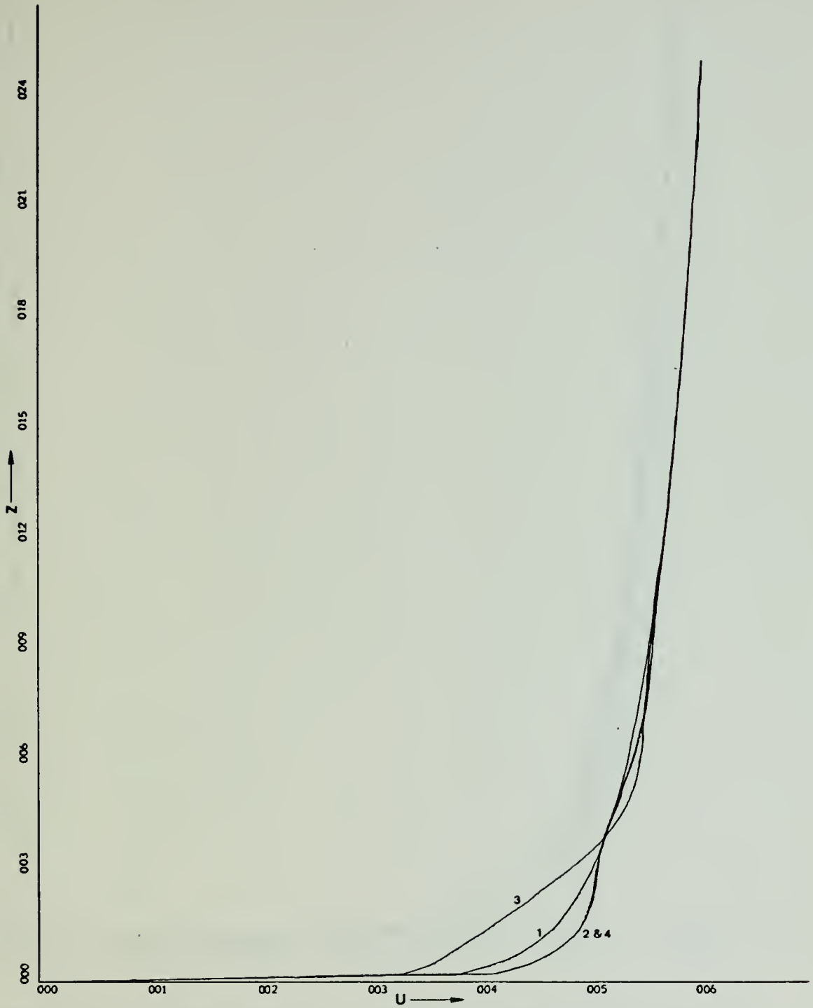
Figure 9. Distribution of the mean wind velocity ( U in \text{m sec}^{-1} ) with height ( z in meters) for wave number ( k ) equal to 0.0400 \text{ m}^{-1} . Comparison is made where: 1) initial mean velocity profile; 2) series 4; 3) series 5 and 6; 4) series 7.
