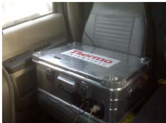
Figure 6. Removable Mobile System and Display/Mapping Unit (Can be deployed in vehicle, boat, or helicopter)
