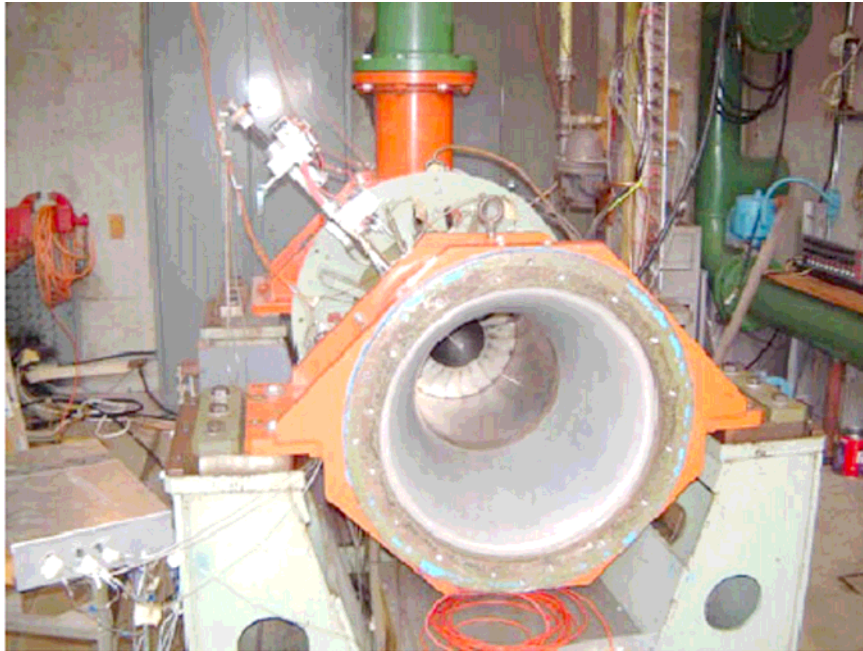
Figure 2. Transonic compressor rig in test cell with inlet piping removed.
