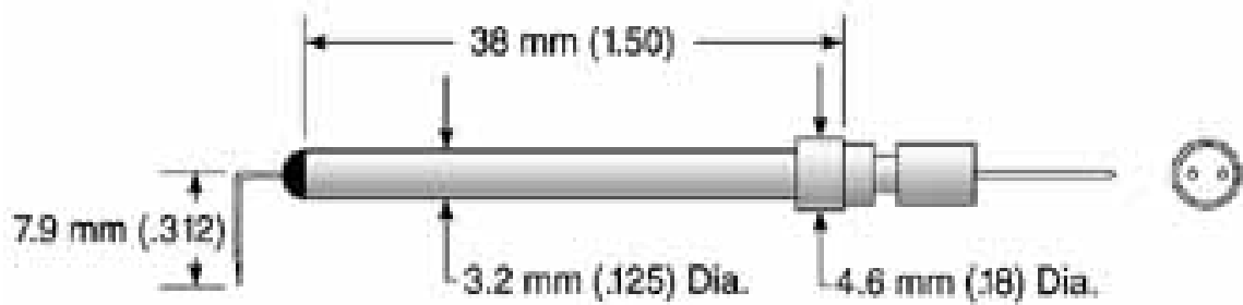
Figure 7. TSI model 1212-20 hot-film probe (From Ref 12)
