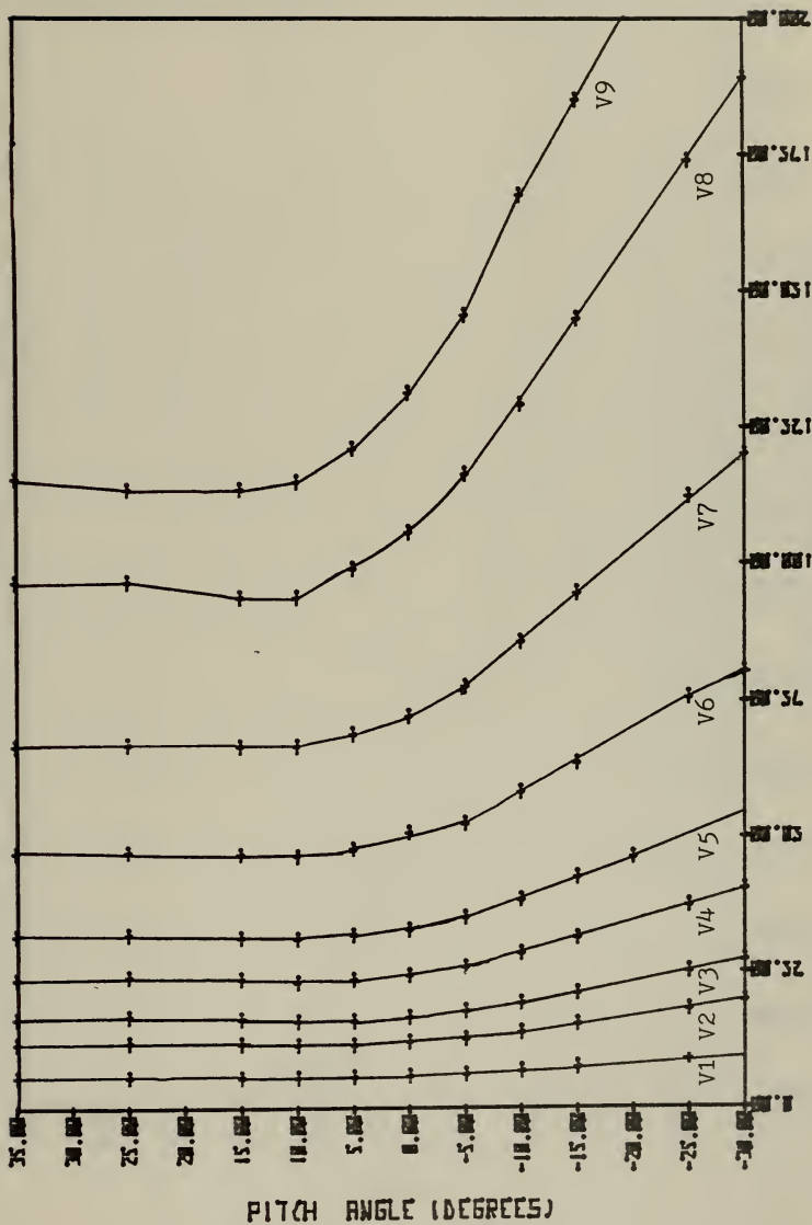
FIG. 10 . (PI-P23) VS. PITCH ANGLE FOR NINE VELOCITIES.
