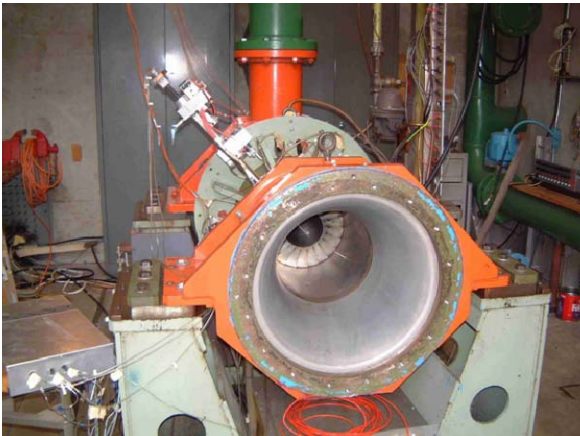
Figure 3. Transonic compressor rig in test cell with inlet piping removed.
