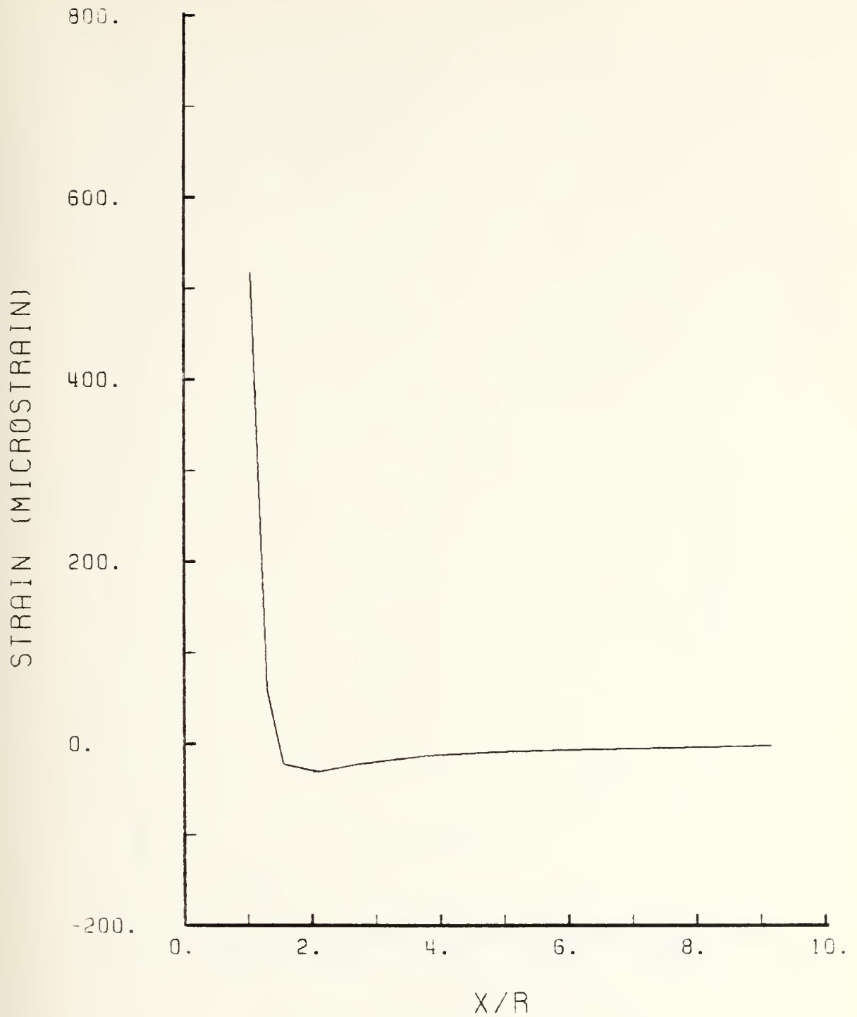
Figure 23. Computed \epsilon_{xz} Vs X/R Unreinforced Panel.
