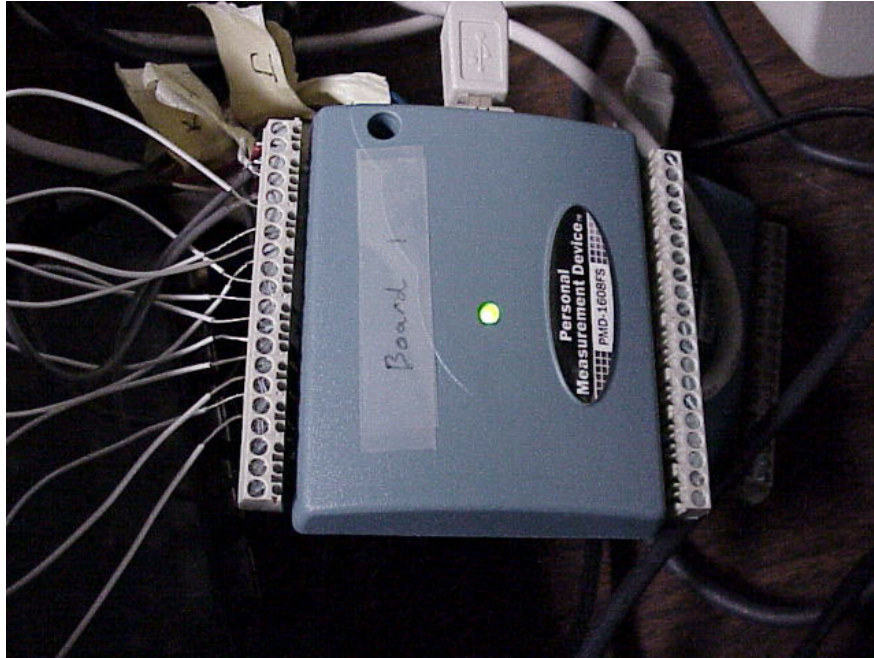
Figure 11. PMD-1608FS analog and digital I/O module
