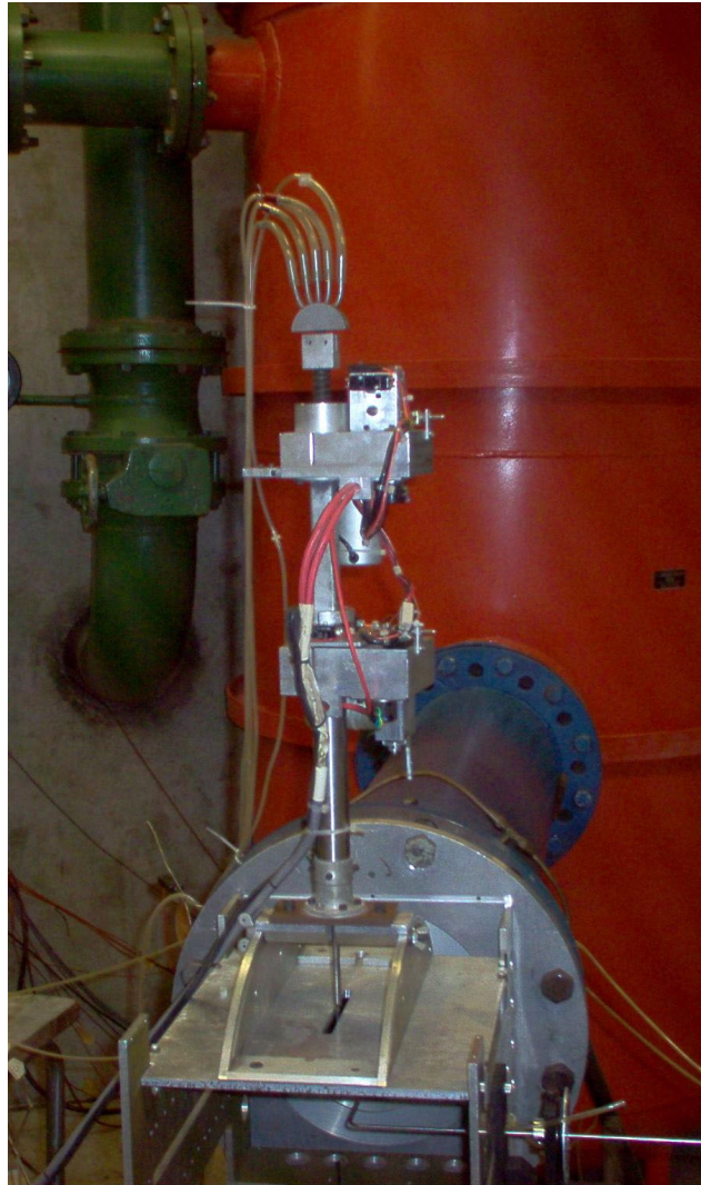
Figure 8. L.C. Smith probe actuator mounted on the free-jet rig
