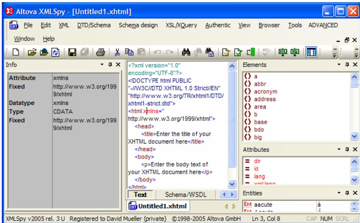
**Figure 3. Altova XMLSpy gives information about the element currently being edited on the left side of the application window. [Altova 2005]**
