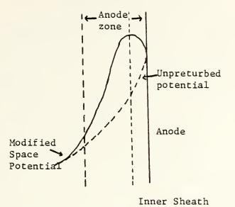
Fig. 5 Potential distribution due to positive space charge build up caused by a local plasma pressure increase.
