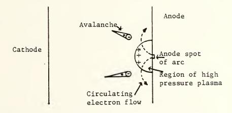
Fig. 6 Circulating electron flow in region of high pressure plasma at the anode.
