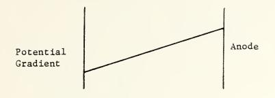
Fig. 3 Linear potential gradient across the working medium of a CO<sub>2</sub> laser.
