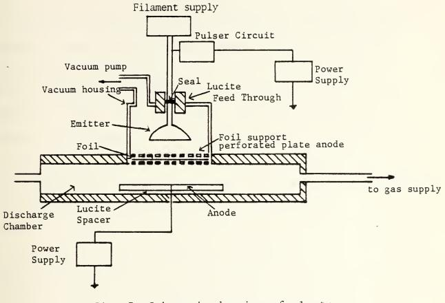
Fig. 7 Schematic drawing of electron beam sustained discharge.
