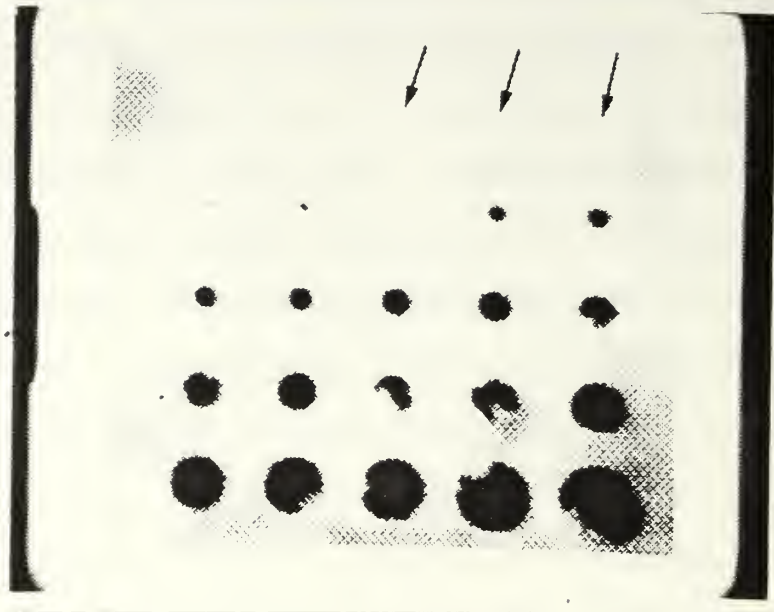
Figure 4.7 White Light Calibration Array Image Showing the Three Smallest Features (Arrows)
