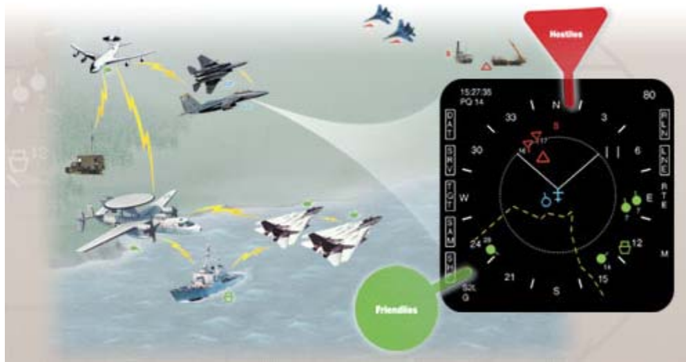
Figure 37. Link 16 provides highly accurate position data and identification of friend or foe (IFF). 78
