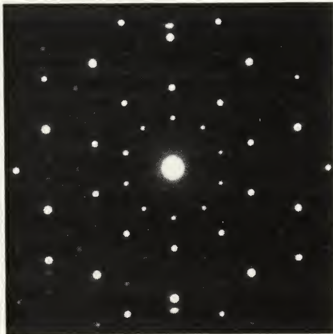
Figure 17. (a) Higher magnification TEM micrograph of particle identified in the previous figure. Note blocky morphology and large (1-2 \mu\text{m} ) size. (b) Characteristic five-fold symmetry identifying the particle as T_2 .
