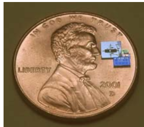
Figure 3. Solar powered, bi-directional communications & sensing (acceleration, ambient light) (From Ref. 8).
