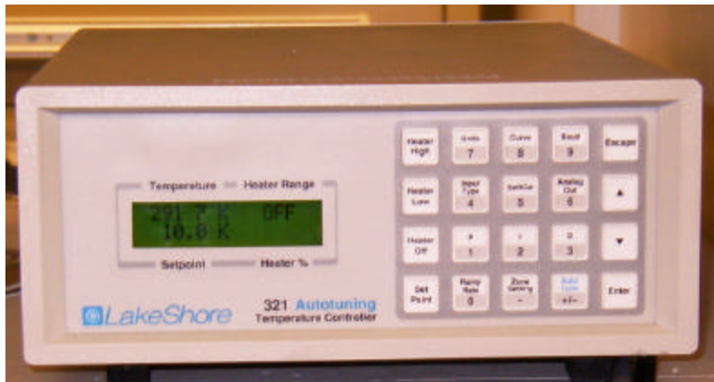
Figure 20. LakeShore 321 Autotuning Temperature Controller set to 10K.
