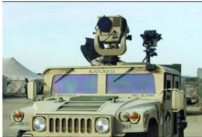
Figure 9. M1114 with a pedestal mounted LRAS3<sup>35</sup>
