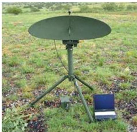
Figure 11. AN/PPS-5D Ground Surveillance Radar<sup>40</sup>
