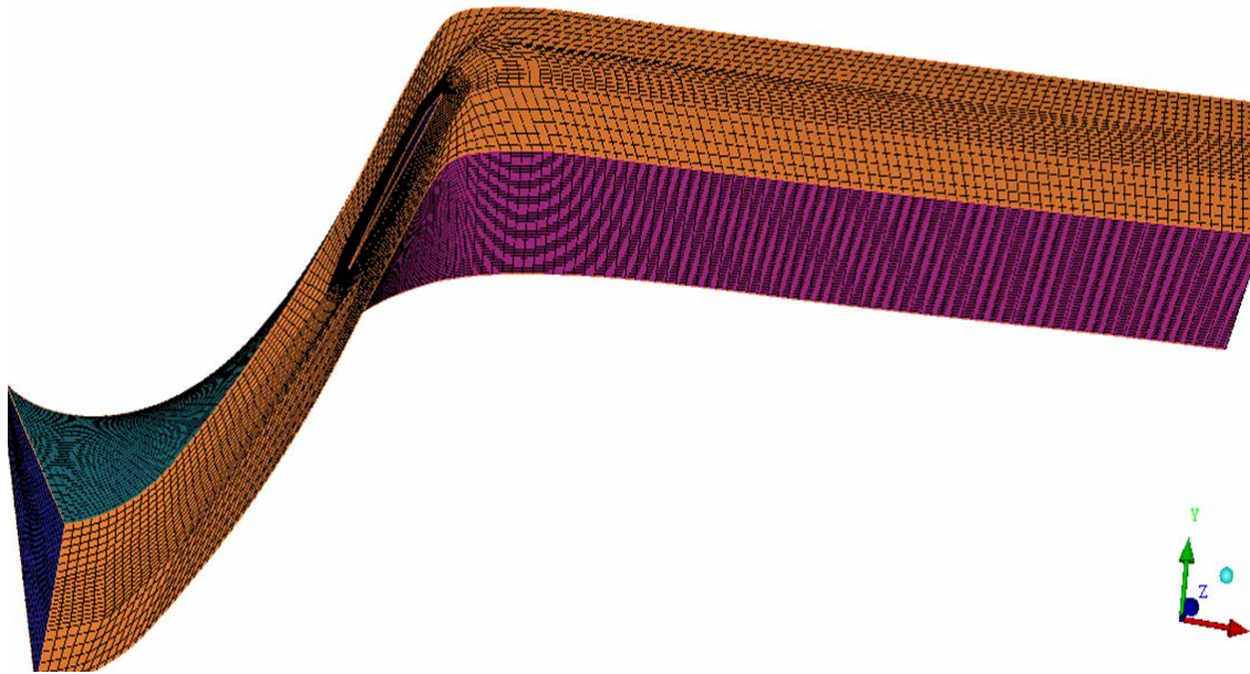
Figure 15. Hub Assembly Mesh Created in ICEM-CFD
