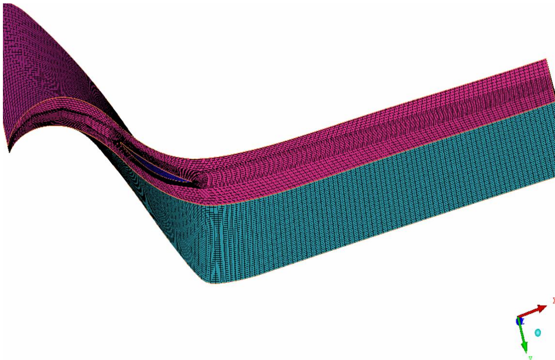
Figure 16. Shroud Mesh Created in ICEM-CFD
