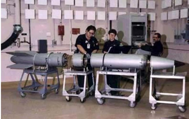
*Technicians maintaining a B-61 gravity bomb. This nuclear munition has been identified as one that could be modified to hit hardened underground targets.*
