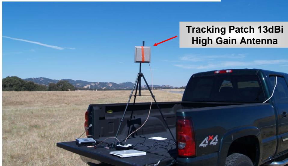
Figure 9. UAS Ground Rehearsal Antenna Set-Up
