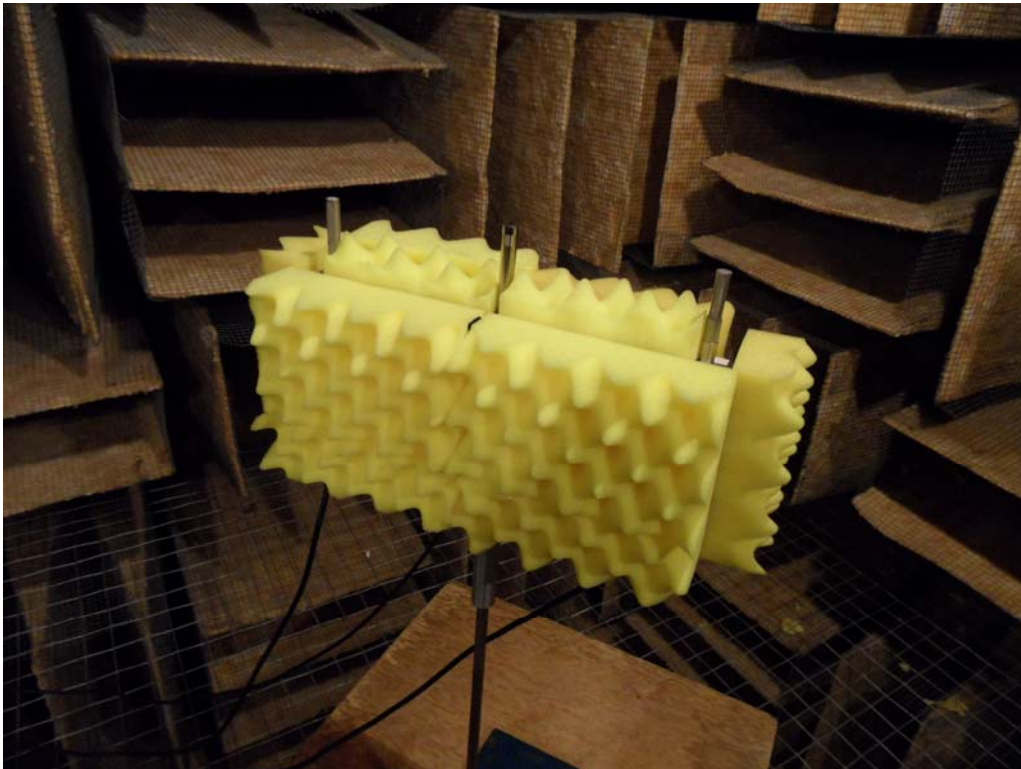
Figure 12. Foam padding to minimize reflection from holder
