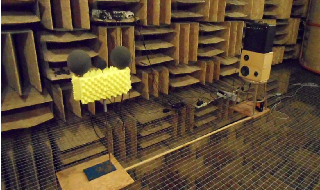
Figure 13. Positioning of noise source for BLUE MRA measurement (shown with windscreen attached)
