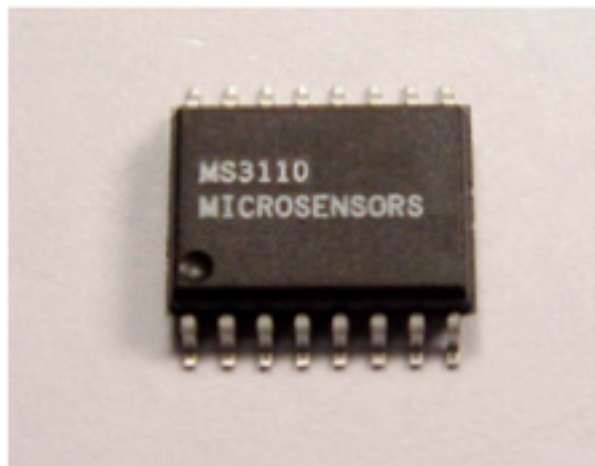
Figure 10. Here a close up view of the MS3110 16-Pin SOIC is presented (From [11]).
