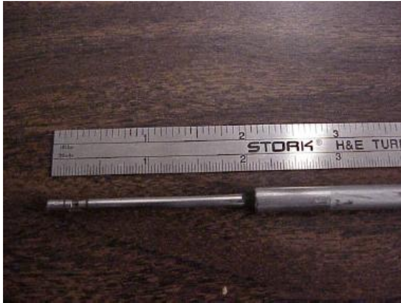
Figure 7. Five-hole probe [From Ref. 2]
