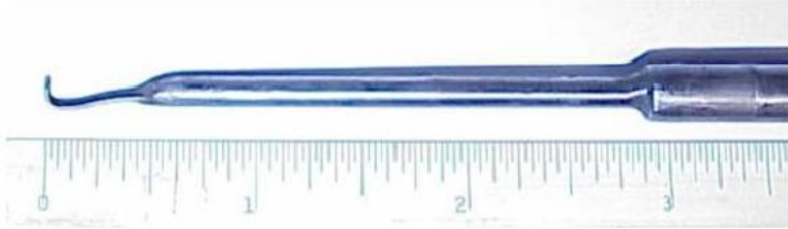
Figure 9. Three-hole cobra probe [From Ref 12]
