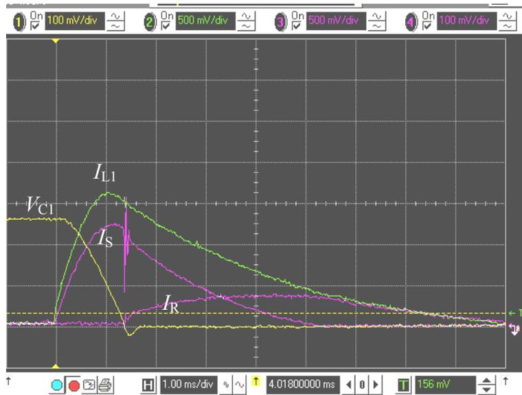
Figure 15. Preliminary Testing, Counterpulsing With No Opening
