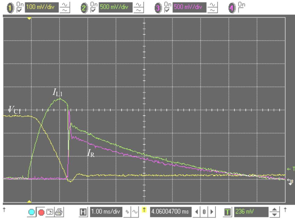
Figure 14. Preliminary Testing, Opening With No Counterpulse
