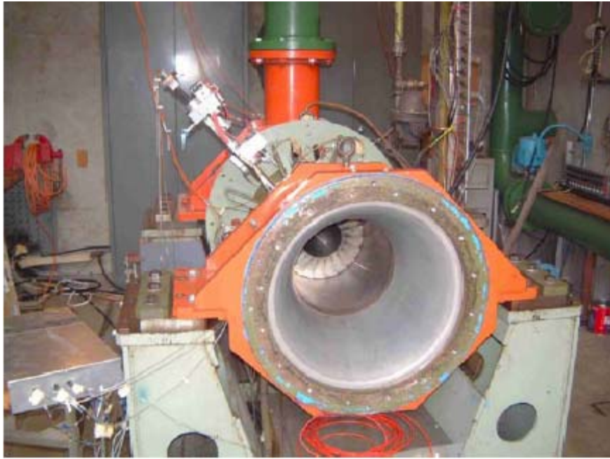
Figure 3. Transonic Compressor in test cell with inlet piping removed (From Ref. 8)
