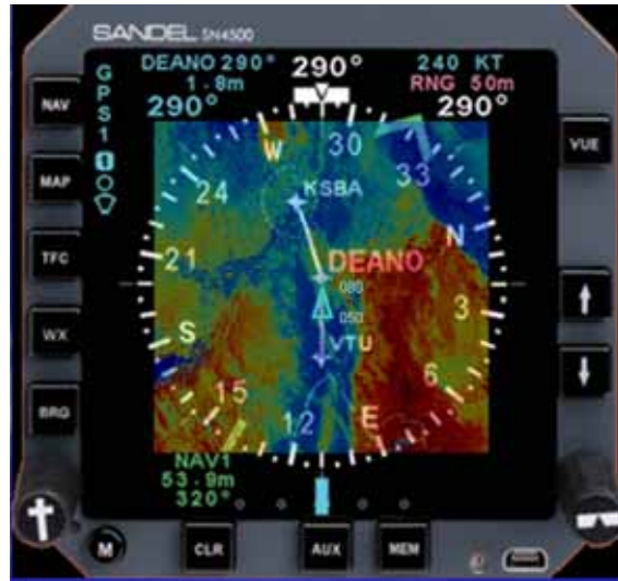
Figure 3. A typical depiction of a standard EHSI with a MODIS based icing potential overlay (sandel.com 2006)
