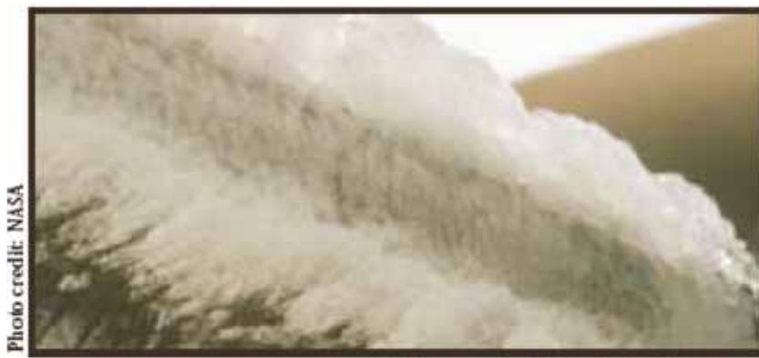
In-flight wing leading edge ice formation
