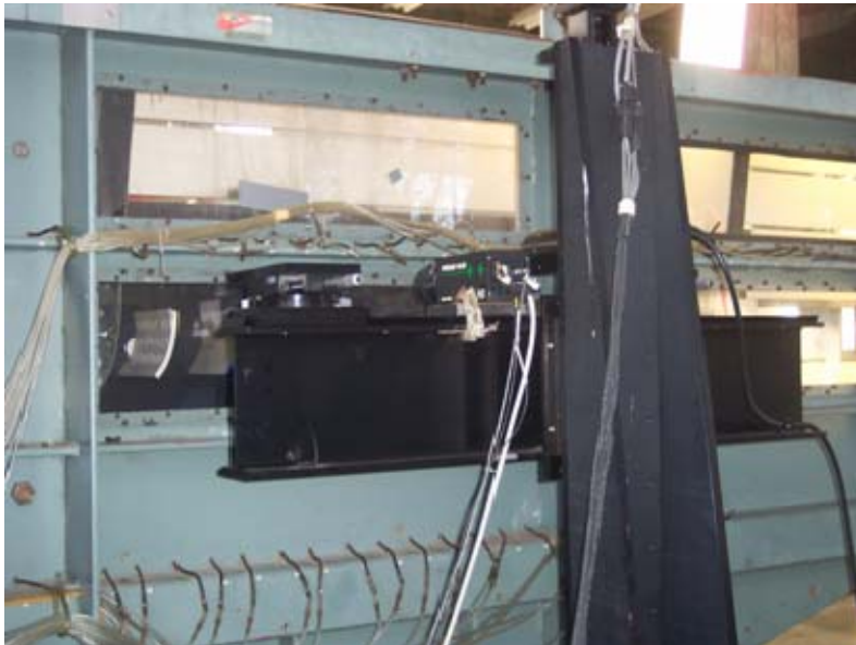
Figure 7. TSI camera mounted on the LDV mechanism.
