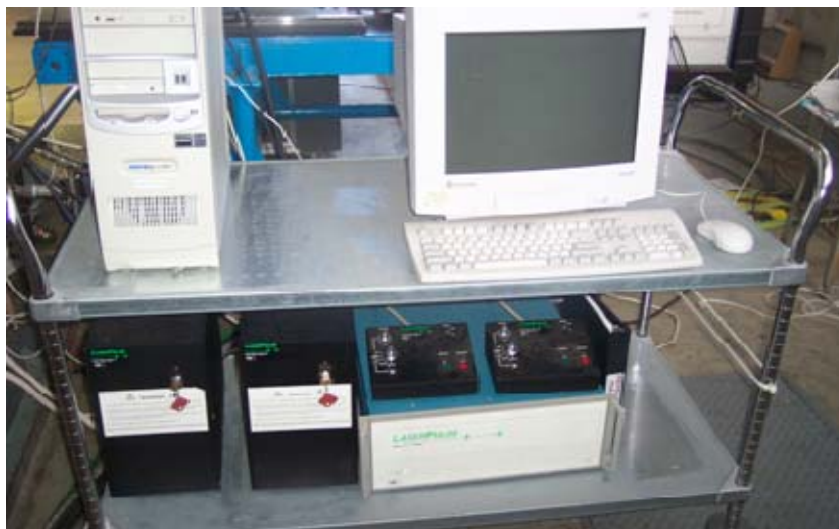
Figure 5. Part of the PIV system showing the computer, laser power supplies and synchronizer.
