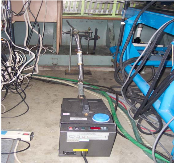
Figure 12. Smoke generator and location of the seeding wand in the LSCWT.
