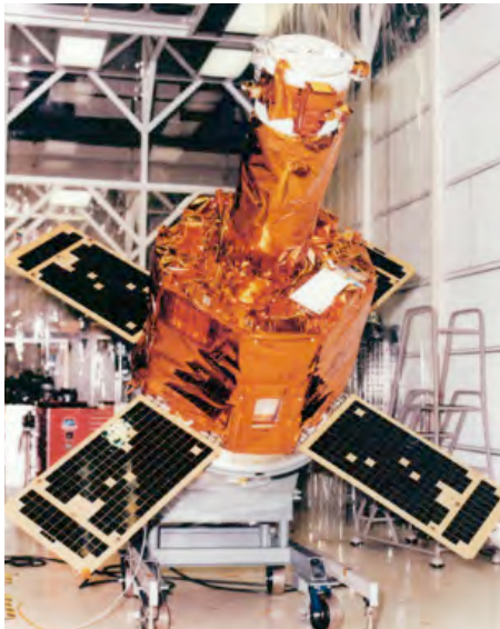
Photograph of the TRACE spacecraft undergoing pre-launch checkout at NASA.
