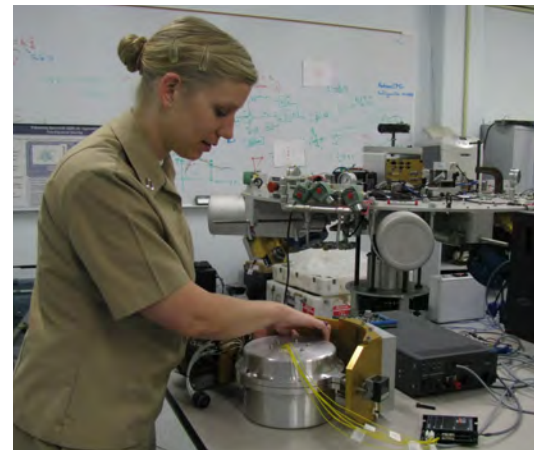
LT Kerri Ackman working on the control moment gyroscope she designed and built as part of her recent M.Sc. thesis. This hardware will be used to evaluate new attitude control systems for agile spacecraft.
