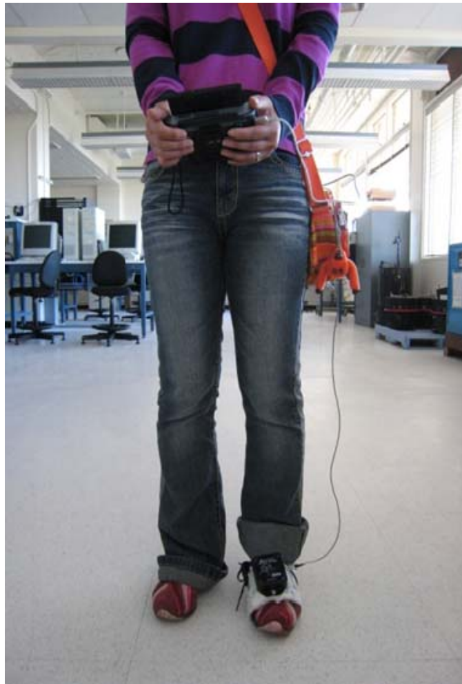
Figure 9. MARG Sensor Attached to a Foot and Connection with a Computer and Battery.
