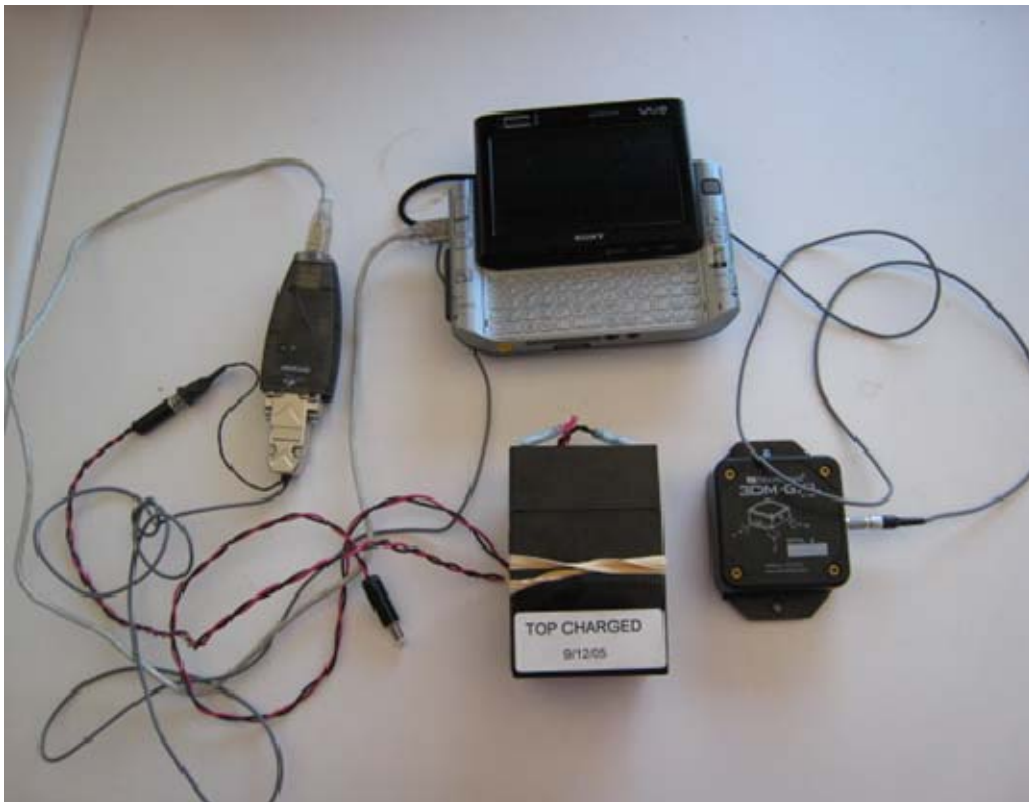
Figure 8. MARG Sensor with Peripheral Equipment for Operation.
