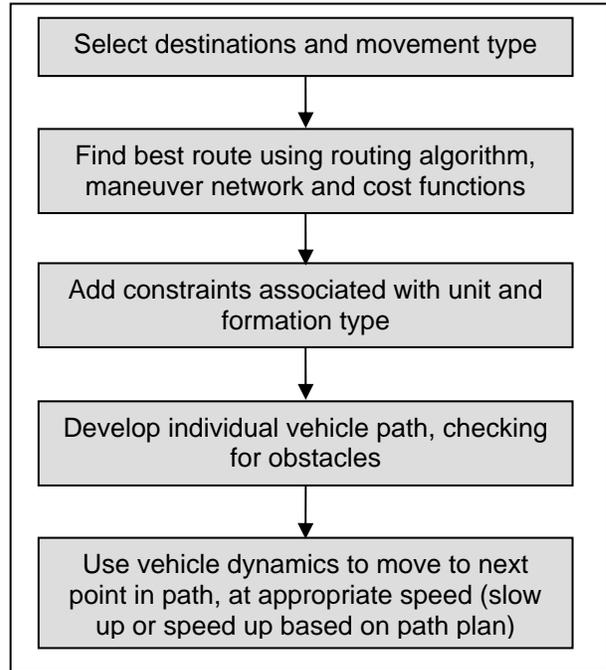
Figure 2.4.1. Common Elements in Maneuver of Ground Vehicles in a SAF Simulation [5].
