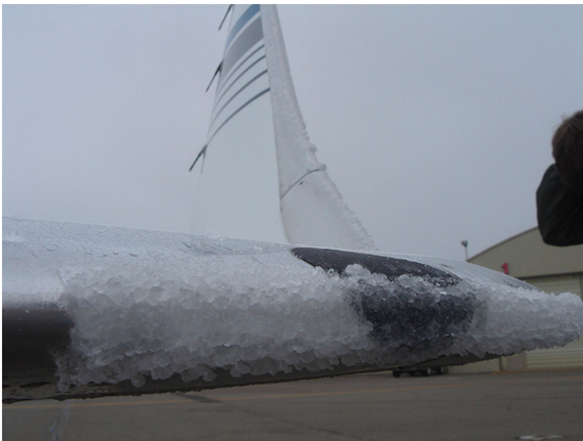
Figure 1. Ice accreted on wing from (From Hearn 2007)
