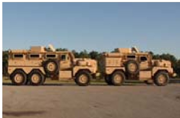
Figure 17. FPII Cougar Vehicles (CAT II and I, respectively) (Force Protection Industries, Inc., 2008)
