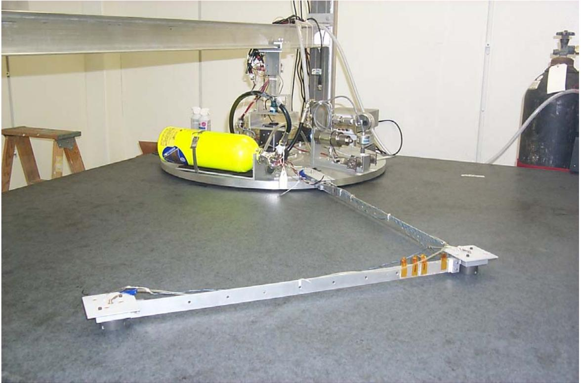
Figure 1. Flexible Spacecraft Simulator FSS)
