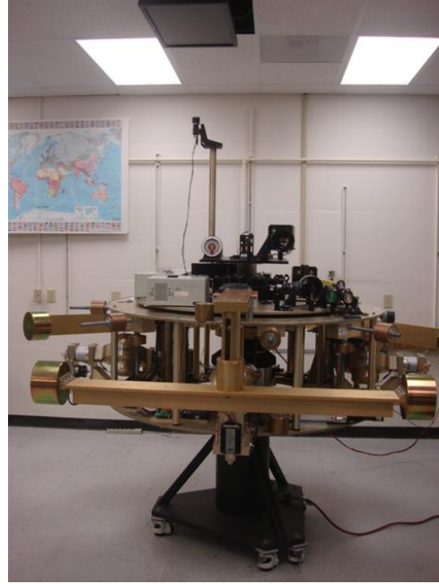
Figure 1. Three Axis Spacecraft Simulator testbed with star tracker camera sticking out the top. LCD monitor suspended in the ceiling displays the star field image.
