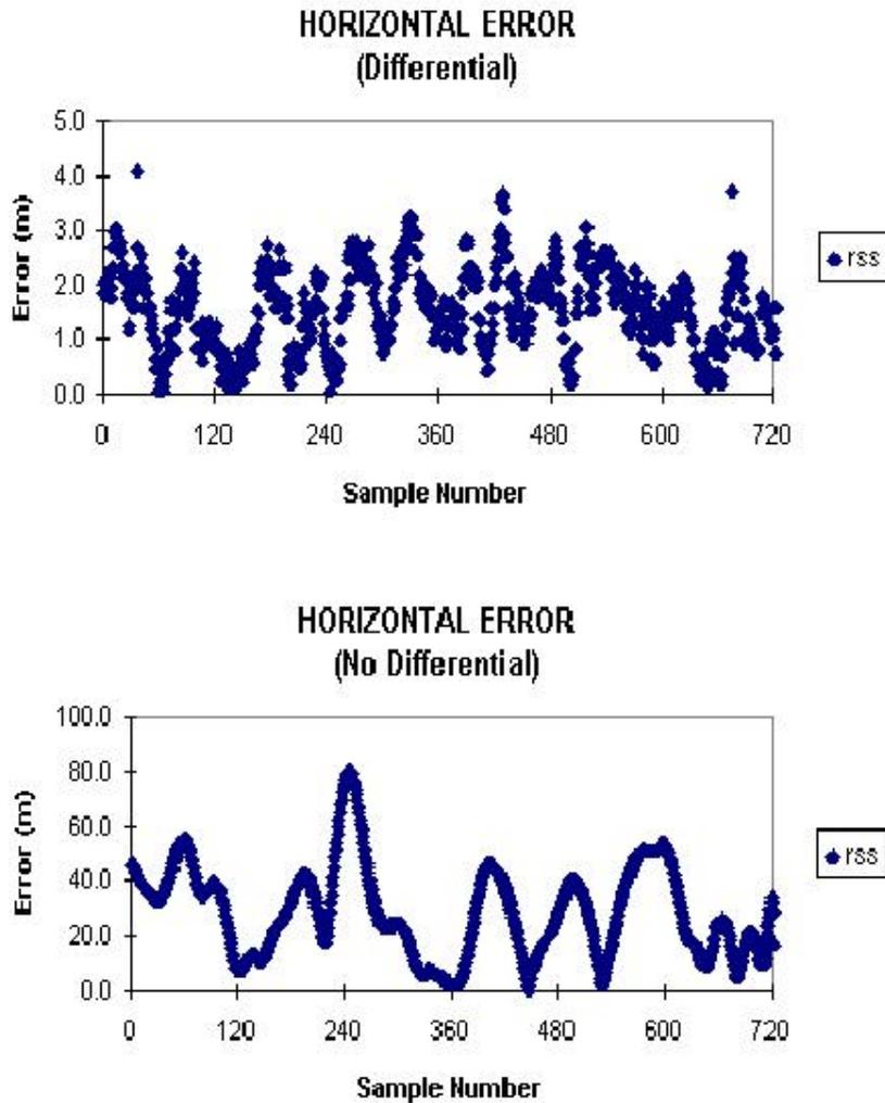
Figure 5: Typical GPS Bench Test Results Recorded over one hour at 5 second intervals
