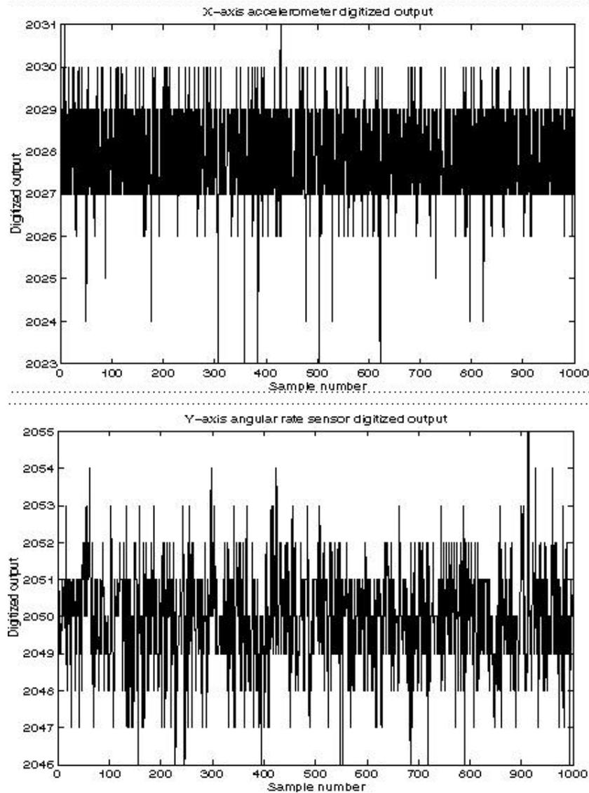
Figure 4: Typical IMU Bench Test Results Recorded Over 83 Seconds at 12Hz Data Rate
