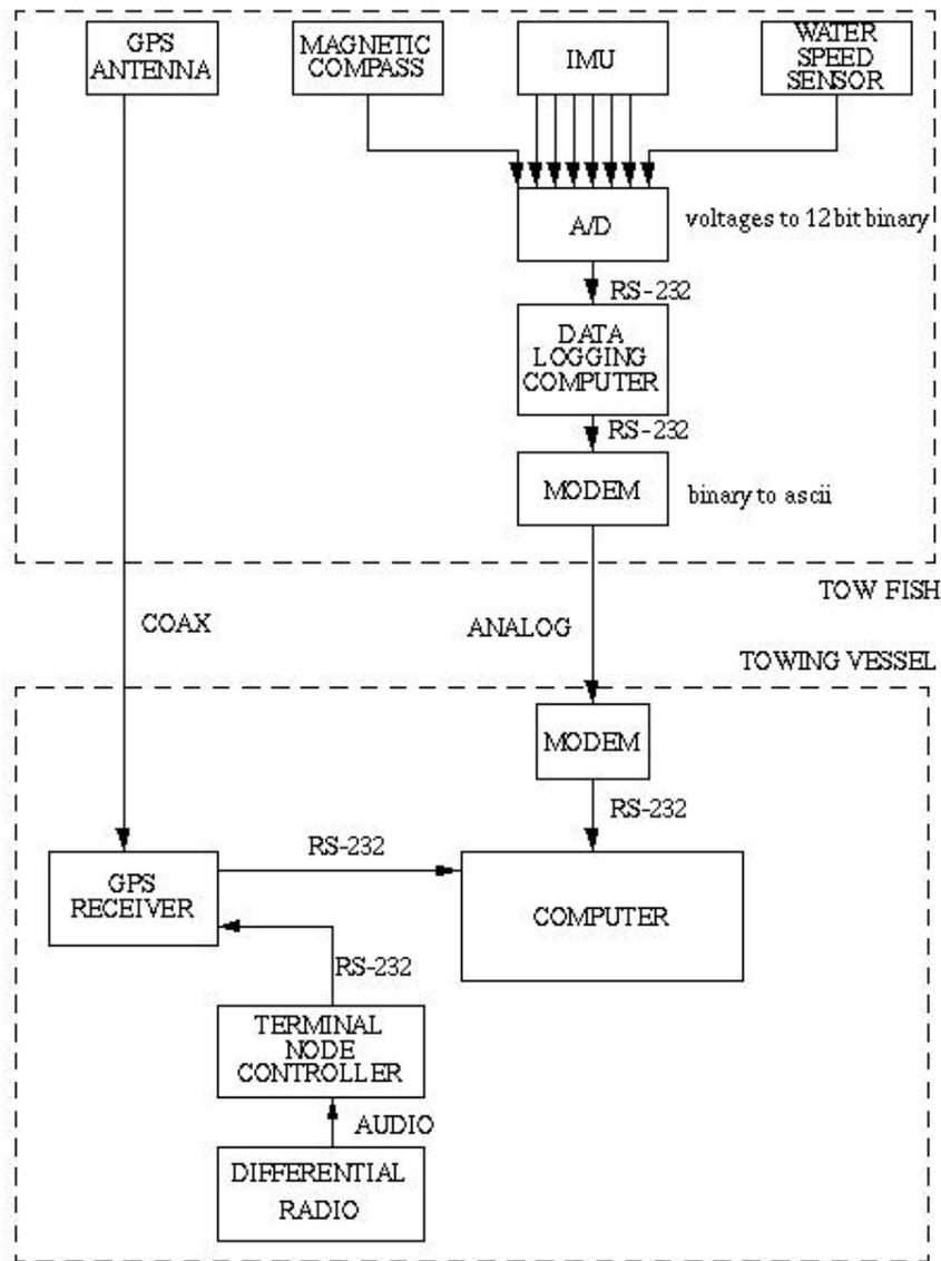
Figure 1: Towfish Experiment Hardware Configuration
