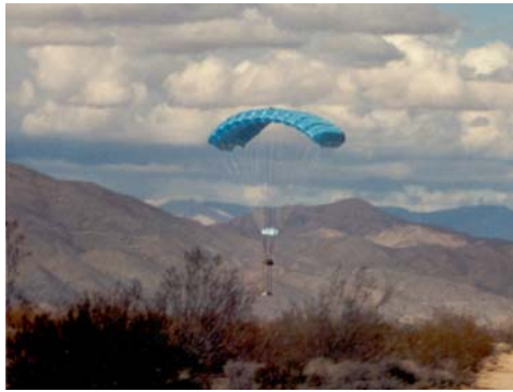
Figure 4. Double-skin 650ft 2 Pegasus parafoil with 500lb payload.
