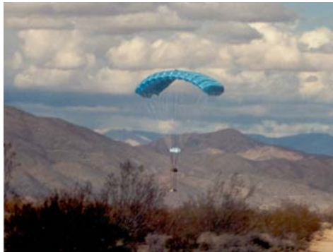
Figure 4. Double-skin 650ft 2 Pegasus parafoil with 500lb payload.
