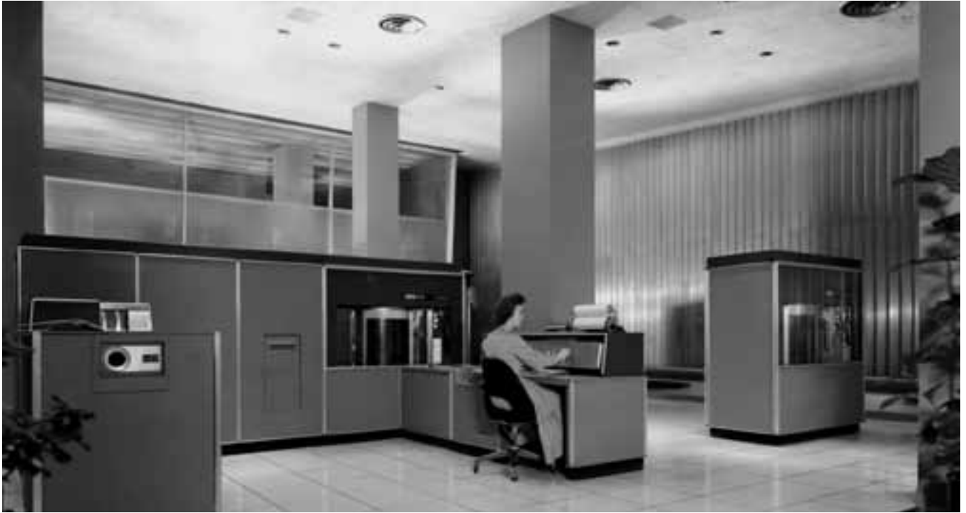
Figure 1. In 1956 IBM introduced the world's first magnetic disk information-storage system, the RAMAC 350 (shown above). A promotional film for the machine showed hallways of file cabinets with frazzled secretaries walking along them. The RAMAC 350, the film showed, stored the entire content of the cabinets in about 2 cubic yards and allowed near-instantaneous searches of the data. To contemporary viewers, the film also demonstrates that the struggle to make the seemingly abstract concept of information tangible is not new. (Photograph courtesy of IBM.)
