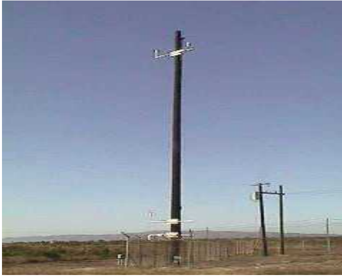
Figure 2. One of 26 Weather Towers located on Vandenberg AFB. Note wind sensors at 2 m and 16 m above ground.
