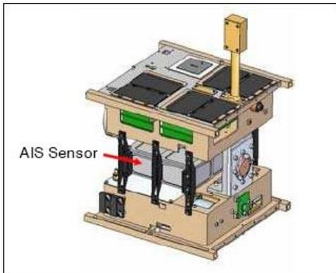
Figure 5: Internal structure of AISSat-1 (Courtesy AISSat)
