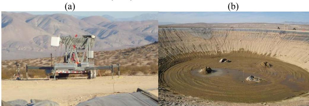
**Fig. 4. (a) High speed digital camera, and (b) GPS for surveying impact holes.**
