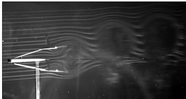
Fig. 10: Centerline wake topology at k = 1.5 .
