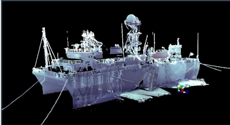
Figure 2. Sample Point Cloud Image (USNS Ship Exterior)
