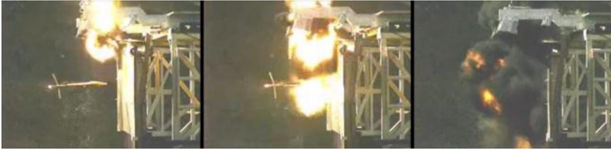
Figure 4. Iron Curtain Sensing, Striking, and Mitigating a RPG Threat
