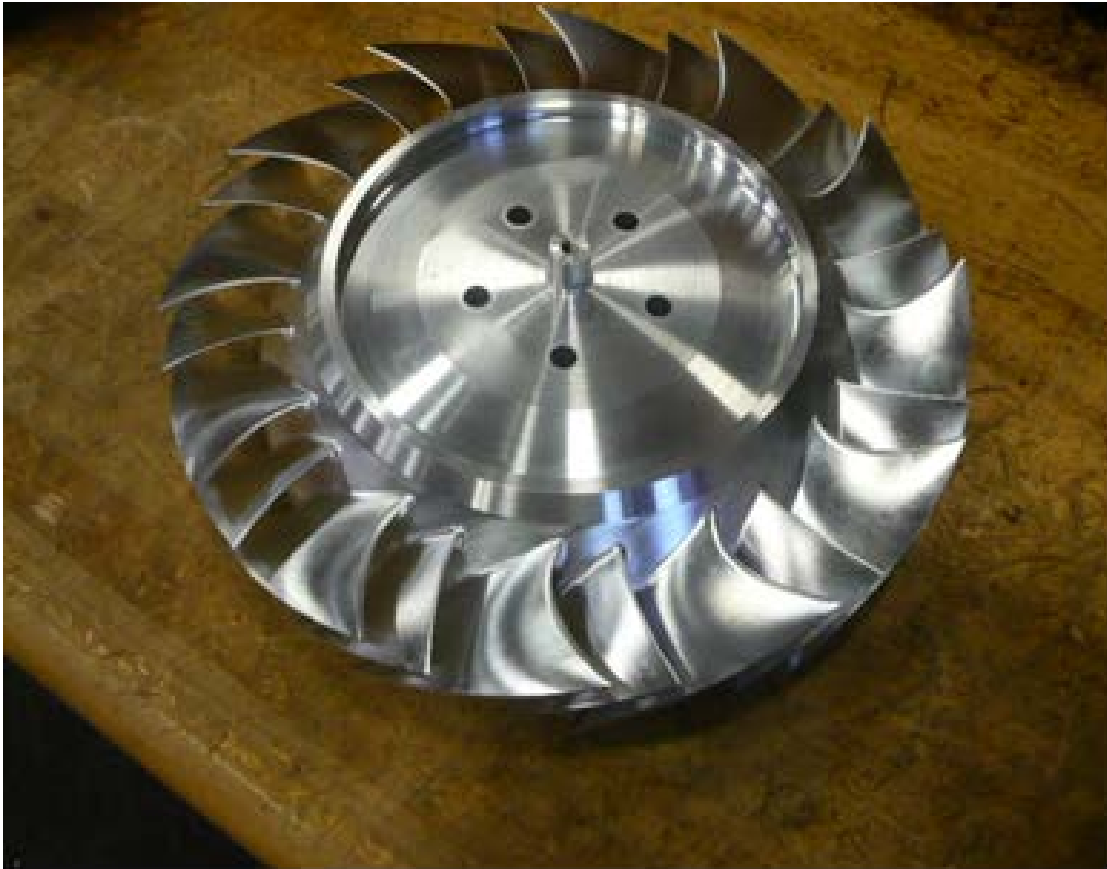
Figure 39. Final machined TASR blisk
