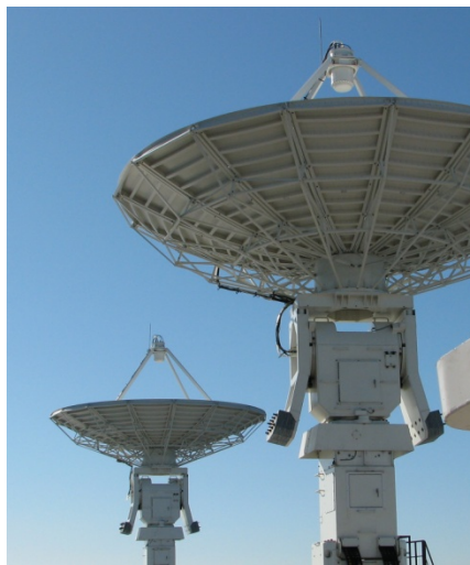
Figure 5. The two 7.3m tracking antennas (with radomes removed) utilized by TTS-1
