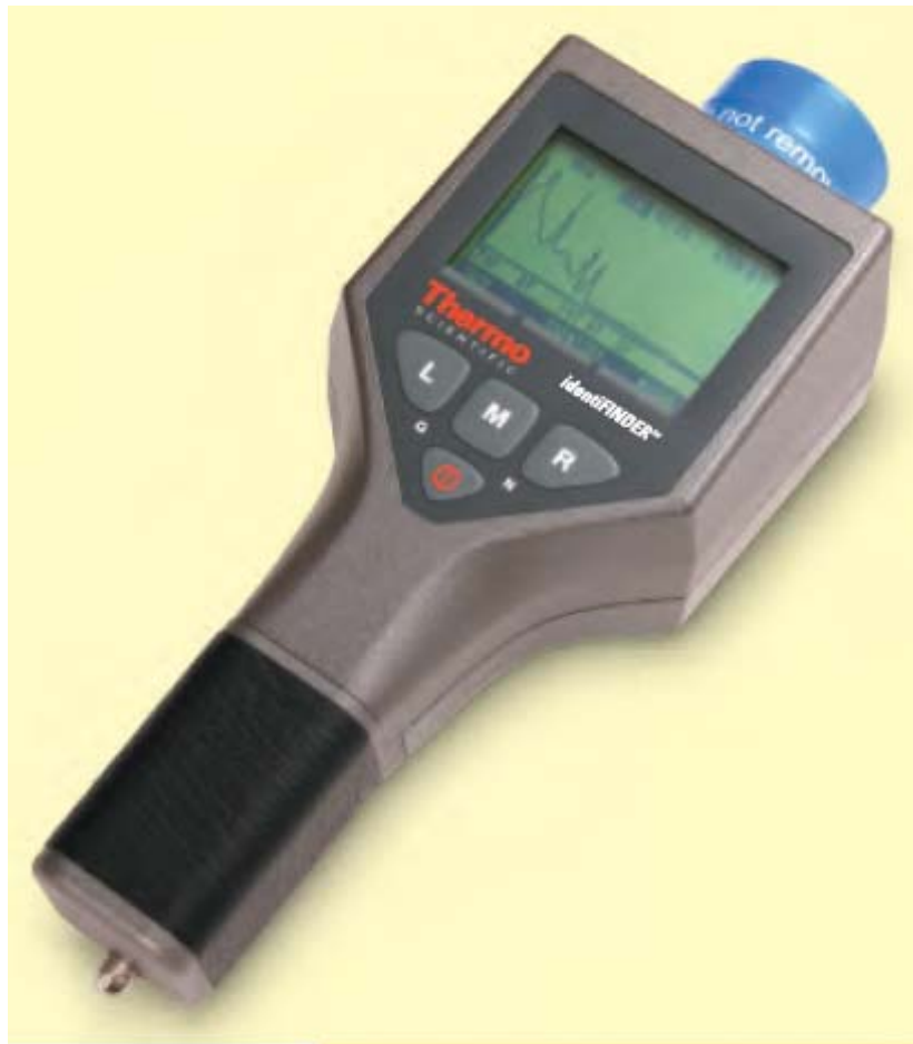
Figure 9. Thermo Scientific Isotope identiFINDER (From Thermo Scientific, 2008)
